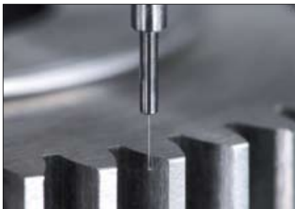
Module 0.8 master gear measurement
