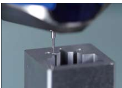
MPP-NANO mold scanning
